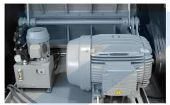
In order to keep the GSC series as compact as possible, motor and hydraulic opening system are integrated into the sound dampening enclosure of the machine.
