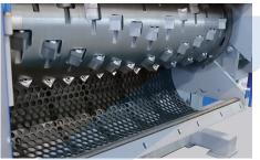
All ZERMA shredders are equipped with a large diameter flat rotor. The knives are fixed in special knife holders fitted in machined pockets. Optional weld on hard facing is available for abrasive applications.
