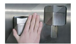
The shredders use concave ground square knives, producing high quality output. The cutters can be turned after a side is worn out.
