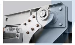
The oversized gearbox driving the rotor is supported by a very sturdy torque arm cushioning the shocks created while grinding.
